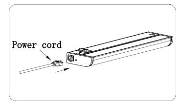
INSTERT LEAD INTO THE INPUT SOCKET. THE INPUT SOCKET IS LOCATED ON The left end of the fixture
