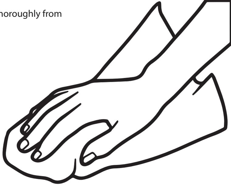
Remove backing from flexible tape. Carefully press the flexible tape to the surface or profile.
